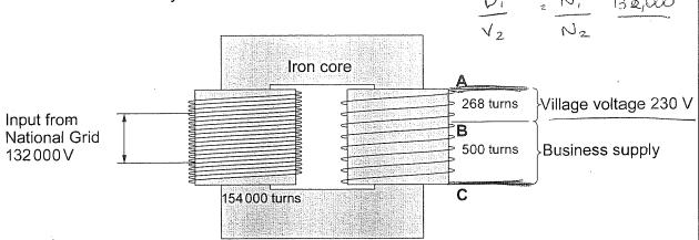
Using an equation from page 2 and information from the diagram calculate the voltage supplied to the business.
