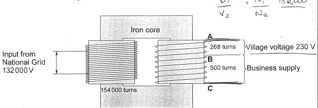
(a) Using an equation from page 2 and information from the diagram calculate the voltage supplied to the business. [3]
